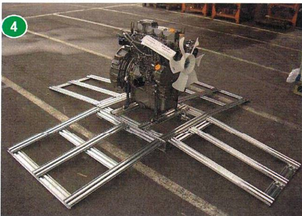
4) Lay side boards down.
